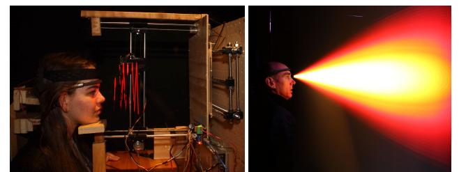
**Figure 4:** Left: Aayinograph of MannLab member Christina, captured with mechanical prototype. Head is stabilized by wooden blocks behind it, and under chin, while stepper motors move a brain-modulated light source through space. Eventually the apparatus will be miniaturized into a wearable device. Right: Interpolated aayinograph™ of MannLab member Steve. Sparsely sampled SSVEP data is interpolated to make the high-resolution aayinograph.
