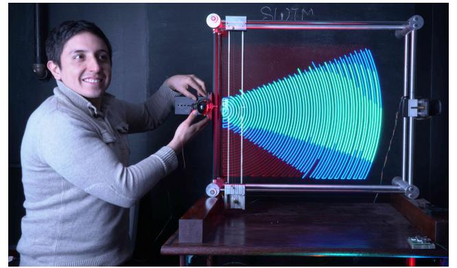
**Figure 6: Metaveilography:** Gear Head USB 2.0 1.3 MP Webcam for PC (WC750RED-CP10). Focus setup at minimum focal length, as expected the picture displays only a limited range of trust region (green). A small defect in the camera is visible near the bottom part of its field of view.
