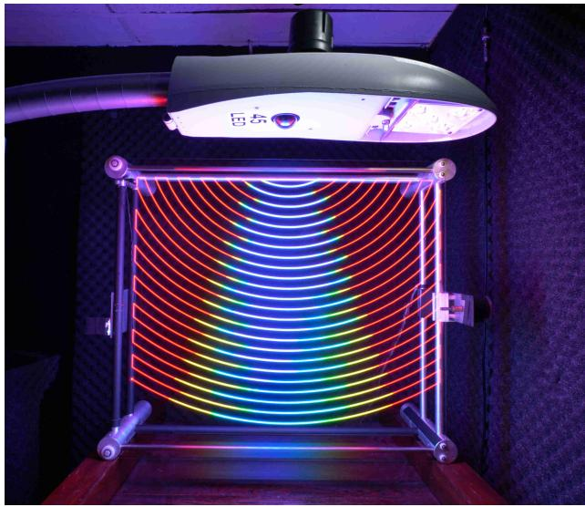
**Figure 7: Unretouched photograph of the smart street light and metaveillographic mechanism showing the streetlight's built in camera and its capacity to sense. Note the slight hysteresis as the light source, moving in circular arcs, is both the sensor as well as the actuator, providing scientific and artistic integrity in the measurement. We can clearly see a physical phenomenon underlying the picture in the form of the hysteresis of even and odd arcs. Compare with figure 3.**
