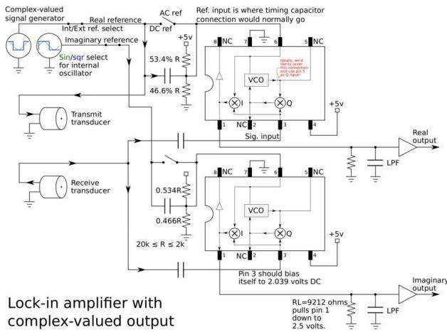
**Figure 9: Schematic of the wearable miniature Lock-in amplifier designed by the authors for a low-cost seeing aid for the blind. See <https://www.instructables.com/member/SteveMann/>**
