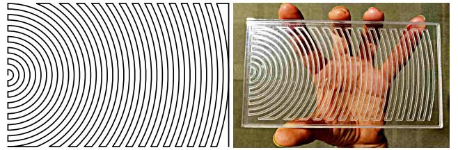
**Figure 8: G-code trial using CNC. The advantage of using G-code is the portability of the code. It can be tested in several different ways. Here the spatial pattern was milled into a block of acrylic and passed around a classroom where metaveillography was being taught.**
