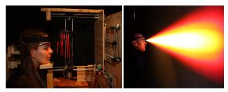
Figure 4: Left: Ayinograph of MannLab member Christina, captured with mechanical prototype. Head is stablized by wooden blocks behind it, and under chin, while stepper motors move a brain-modulated light source through space. Eventually the apparatus will be miniaturized into a wearable device. Right: Interpolated ayinograph<sup>™</sup> of MannLab member Steve. Sparsely sampled SSVEP data is interpolated to make the high-resolution ayinograph.
