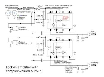
Figure 9: Schematic of the wearable miniaamplifier ture Lock-in designed hv the authors for a low-cost seeing aid for the blind. See https://www.instructables.com/member/SteveMann/
