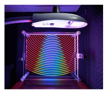
Figure 7: Unretouched photograph of the smart street light and metaveillographic mechanism showing the streetlight's built in camera and its capacity to sense. Note the slight hysterisis as the light source, moving in circular arcs, is both the sensor as well as the actuator, providing scientific and artistic integrity in the measurement. We can clearly see a physical phenomenon underlying the picture in the form of the hysteresis of even and odd arcs. Compare with figure 3.
