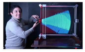
Figure 6: Metaveillography: Gear Head USB 2.0 1.3 MP Webcam for PC (WC750RED-CP10). Focus setup at minimum focal length, as expected the picture displays only a limited range of trust region (green). A small defect in the camera is visible near the bottom part of its field of view.
