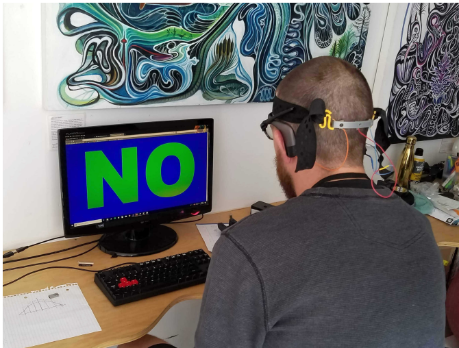
Fig. 7: Experimental setup with observer viewing a displayed image. Here the image is a simple picture of the word “NO” displayed on a dark background. (the image is flickering at 12 Hz).
